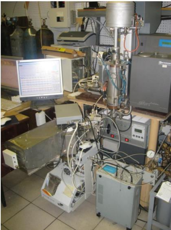
Gas analysis by the GAOS MS-20-8 mass-spectrometer at the thermogravimetric analysis. The installation of TG-DTA/DSC analysis «Setsys Evolution», SETARAM, France. Institute «Gipronickel», Saint-Petersburg, «MMC «Norilsky nickel».
